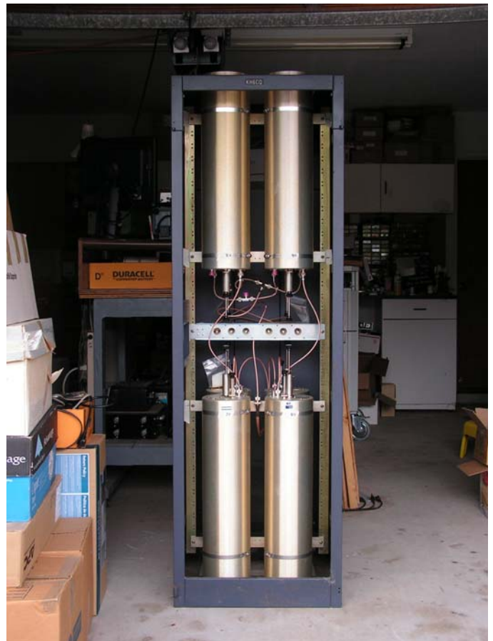
Figure 1 — The two duplexers and band pass cavities mounted in a re-purposed General Electric 19-inch rack cabinet. The front door of the cabinet was removed for this picture.
