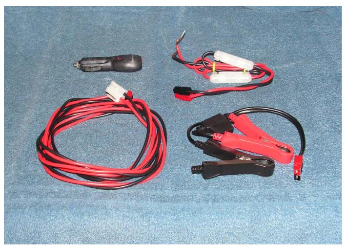
The accessories shown above provide convenient ways to quickly connect your radio to various power sources. Seen clockwise from the upper left are adapters for powering a radio from a vehicle's cigarette lighter socket, an AC power supply, and a storage battery. The cable at the lower left is a factory-supplied power cable that was modified to work with these accessories.
