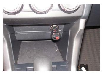
For mobile use, the transceiver's power cord can be plugged into the Powerpole connector on the CigBuddy adapter which plugs into the cigarette lighter socket. This provides an easy way to power the radio from the vehicle's battery; however, you may have to reduce the radio's RF output power (in order to reduce the current drawn by the radio) to avoid blowing the vehicle's fuse. Check your vehicle's owners manual for fuse rating.
