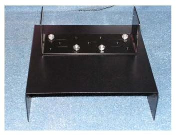
The transceiver's mounting bracket is bolted to the cover of the power supply using short number 10 machine screws, flat washers, and lock washers. Before drilling the holes, check to make sure the heads of the machine screws will not come in contact with any components in the power supply.
