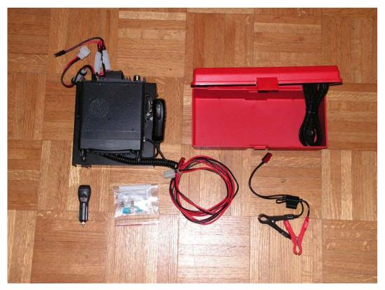
The complete station consists of a transceiver mounted to an AC power supply equipped with a short adapter cable terminated in a Powerpole connector, a CigBuddy, a pack of spare fuses, the transceiver's DC power cord terminated with a Powerpole connector, an alligator clip battery adapter, the AC power cord, and a small box to hold all the accessories.
