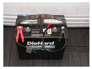
When the transceiver is used as a tactical base station it can be powered by a deep cycle battery and full RF output power can be used if necessary. The alligator clips are placed on the battery terminals and the transceiver's power cord plugs into the Powerpole connector. A 30 Amp in-line fuse is used in this adapter for additional protection. An automotive battery can be used instead of a deep cycle battery in a pinch.
