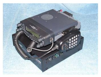
The FM transceiver is mounted directly to the cover of the AC power supply so there is only one unit to carry and stow. When commercial power is available, just plug in the power supply, connect an antenna, and you're on the air.
